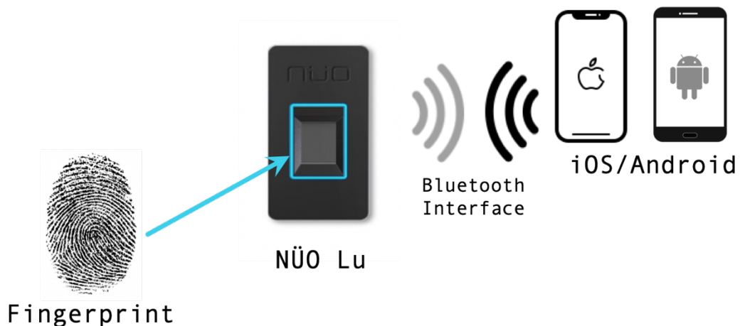
Figure 1. Operational description of NÜO LU reader.
