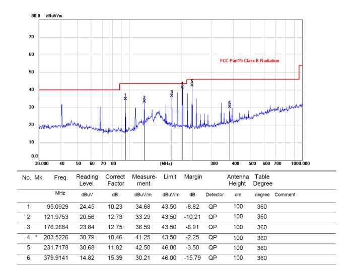
2.Measurement=Reading Level+Correct Factor; Correct Factor=Antenna Factor+Cable Loss.
