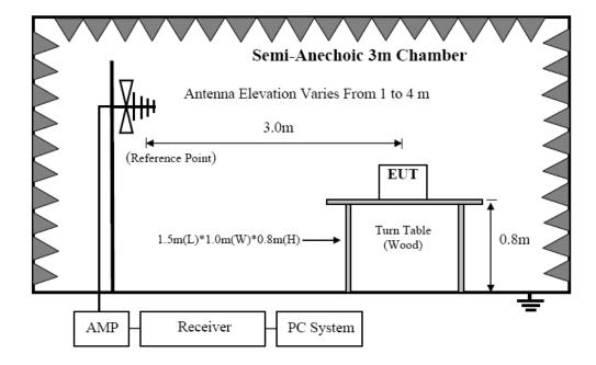
In 3m Anechoic Chamber Test Setup Diagram for frequency 30MHz-1GHz
