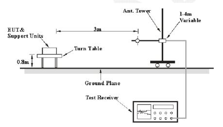
All measurements contained in this report were conducted with ANSI C63.10-2013. The specification used was the FCC Part Subpart C limits.
