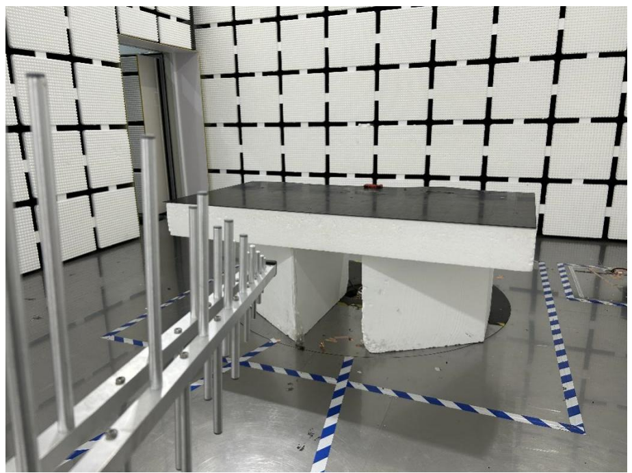
Radiation Emission Test Setup (30MHz to 1GHz)
