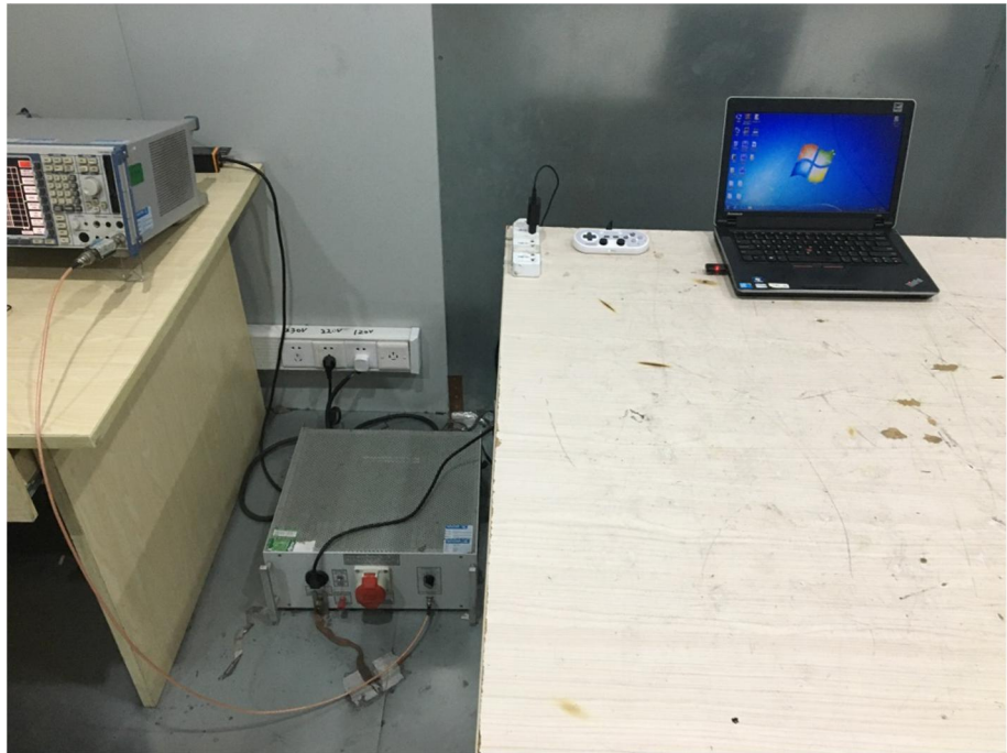
Conducted Emission Test Setup
