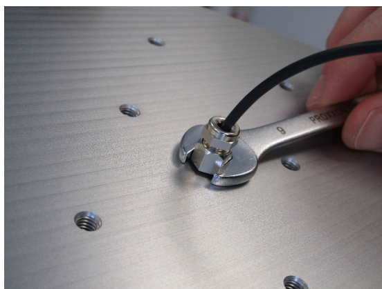
Fig. 8: Securing the M6 cable gland Screw the M6 cable gland into the threaded hole and tighten by hand.
