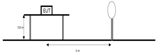
The diagram below shows the test setup that is utilized to make the measurements for emission from 30  $\, \text{Mz} \,$  to 1  $\, \text{GHz} \,$  emissions.
