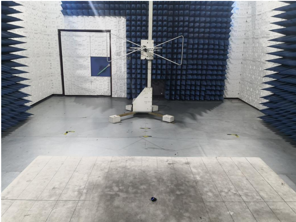
RADIATED EMISSION TEST SETUP ABOVE 1GHZ
