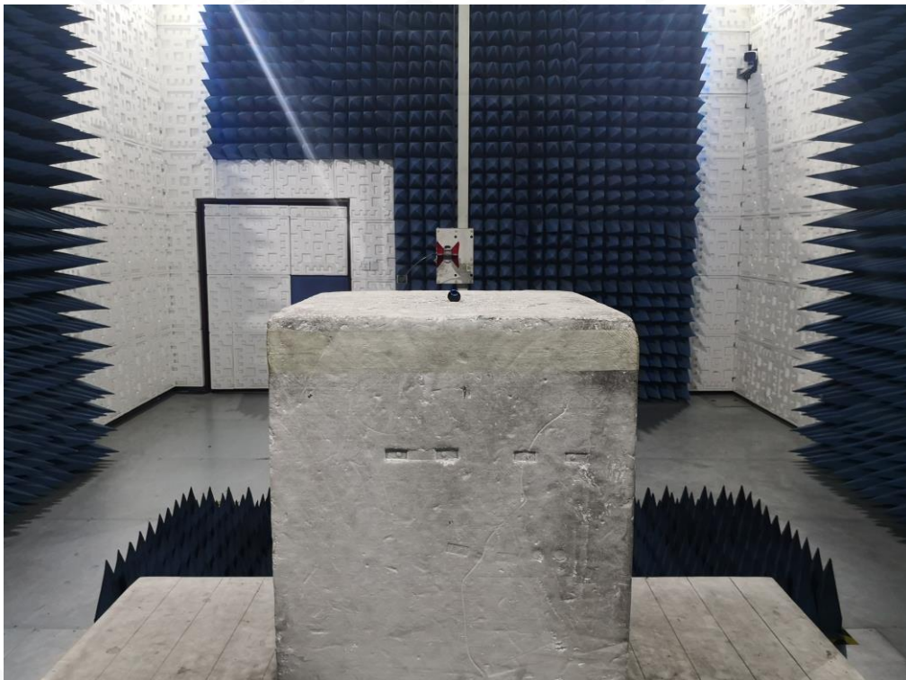
RADIATED EMISSION TEST SETUP ABOVE 1GHZ
