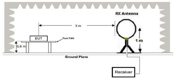
(2) Radiated Emission Test-Up Frequency 30MHz~1GHz
