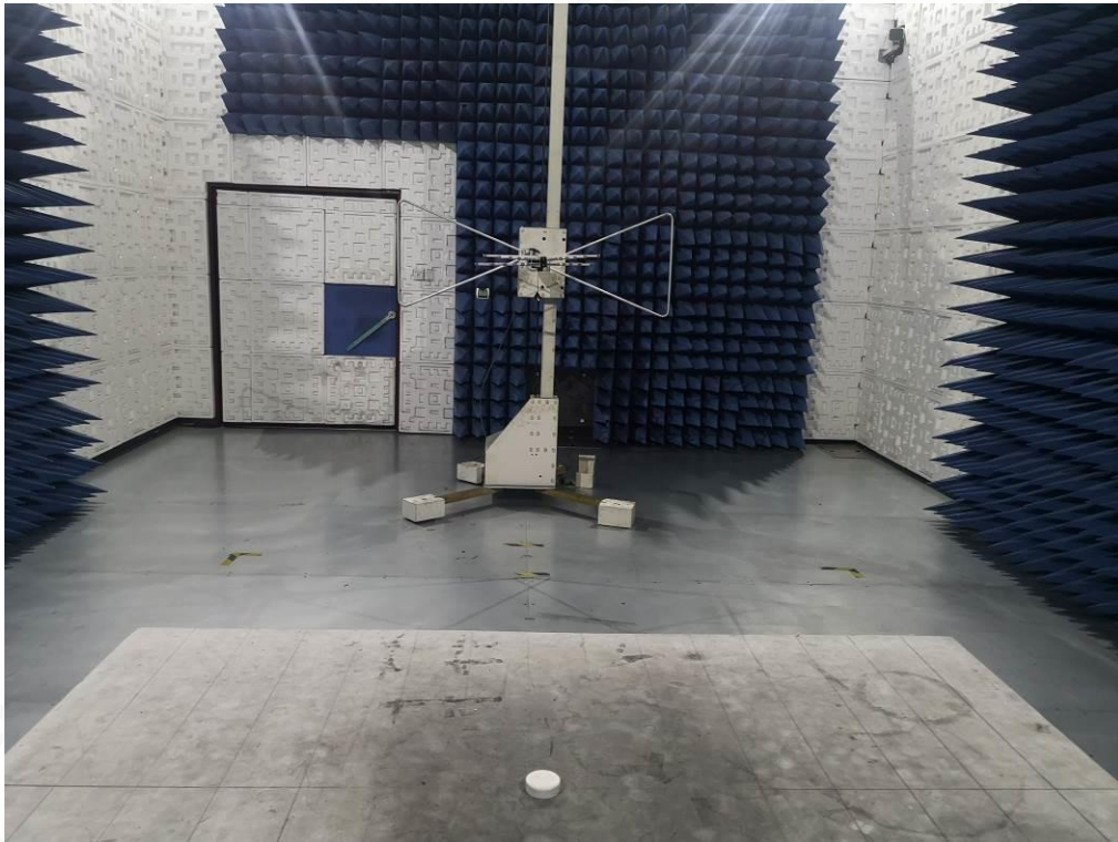
FCC RADIATED EMISSION TEST SETUP-ABOVE 1GHz
