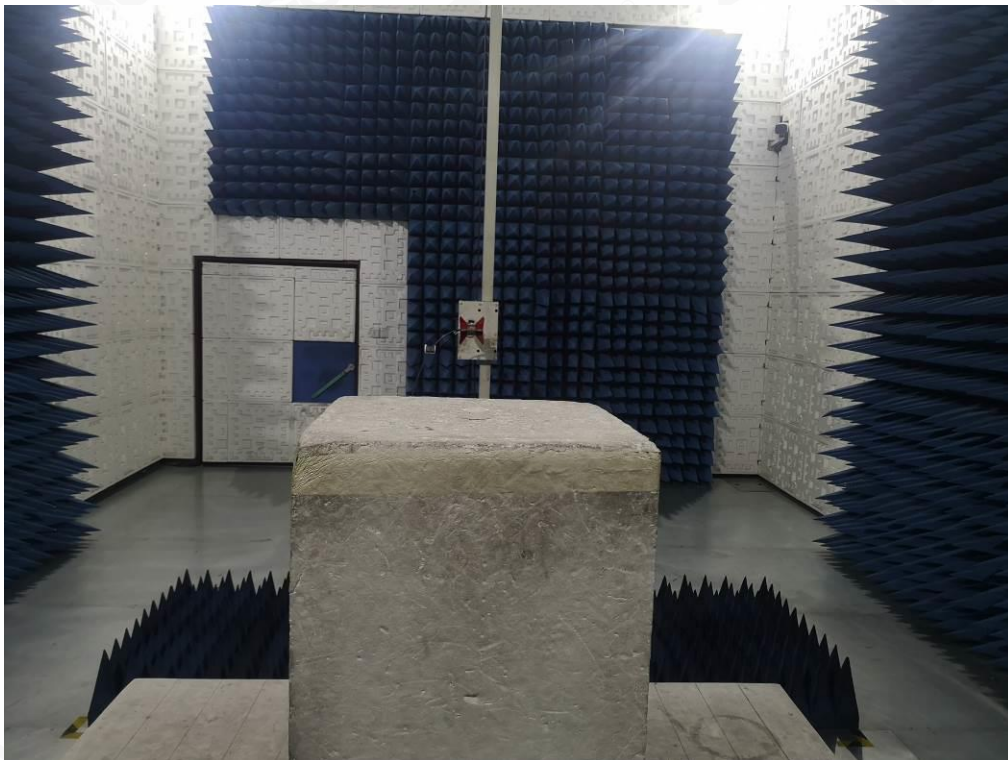
FCC RADIATED EMISSION TEST SETUP-ABOVE 1GHz
