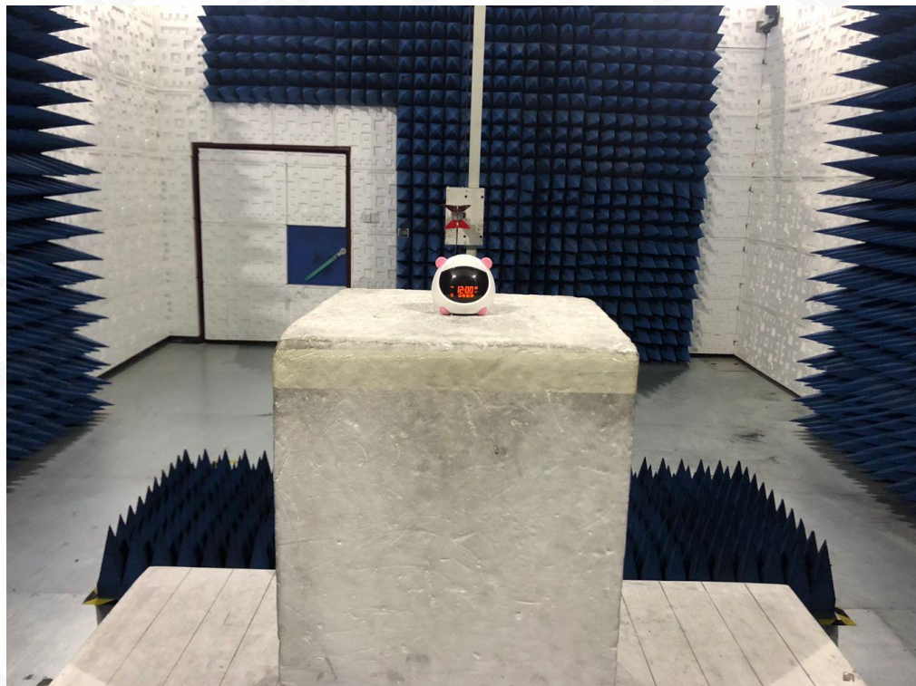
FCC RADIATED EMISSION TEST SETUP ABOVE 1GHZ
