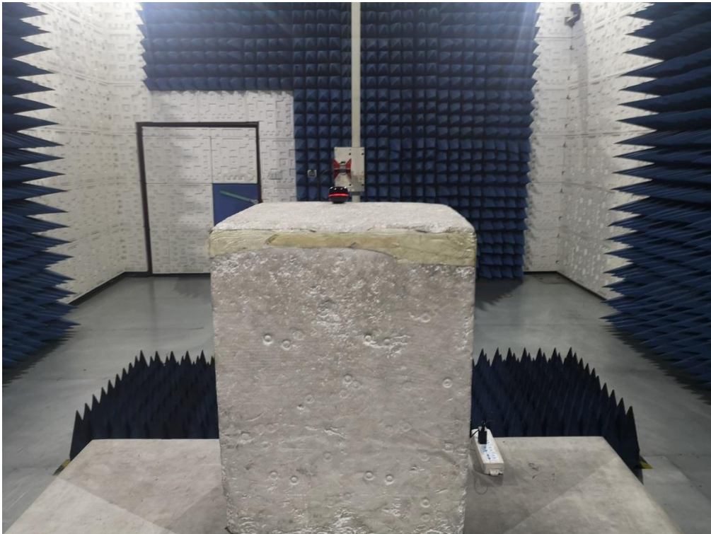
FCC RADIATED EMISSION TEST SETUP ABOVE 1GHZ
