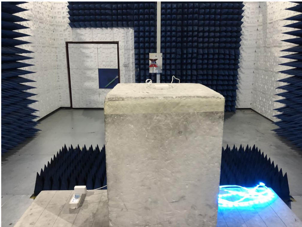
FCC RADIATED EMISSION TEST SETUP ABOVE 1GHZ
