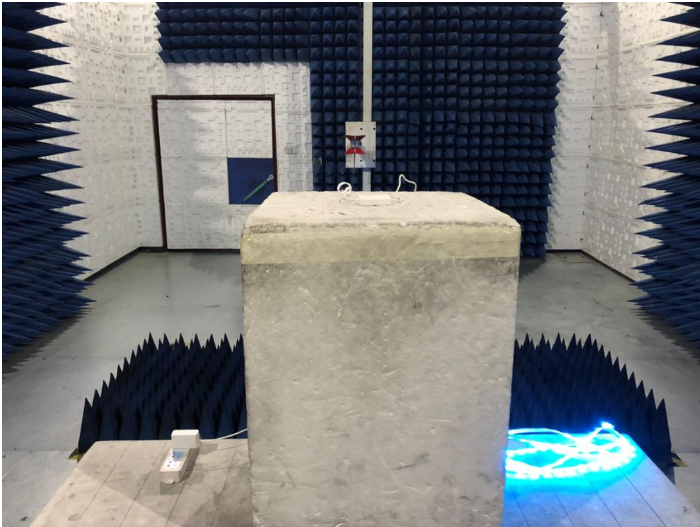
FCC RADIATED EMISSION TEST SETUP ABOVE 1GHZ
