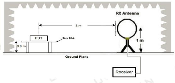
2. Radiated Emission Test-Up Frequency 30MHz~1GHz
