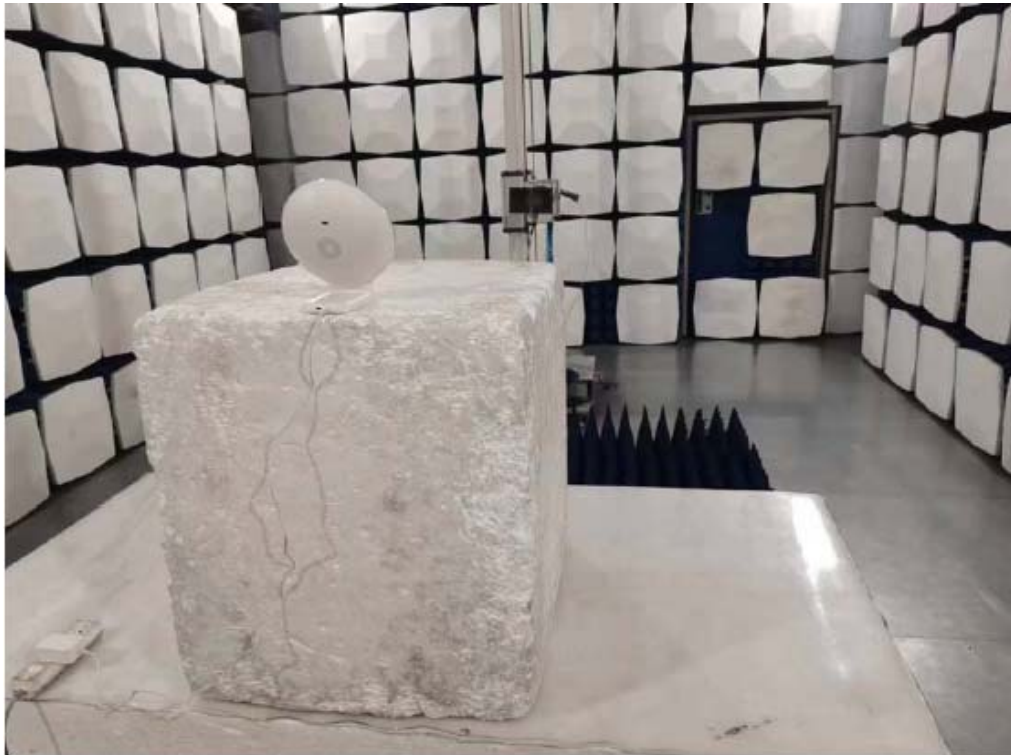
Radiated Emission Test Setup
