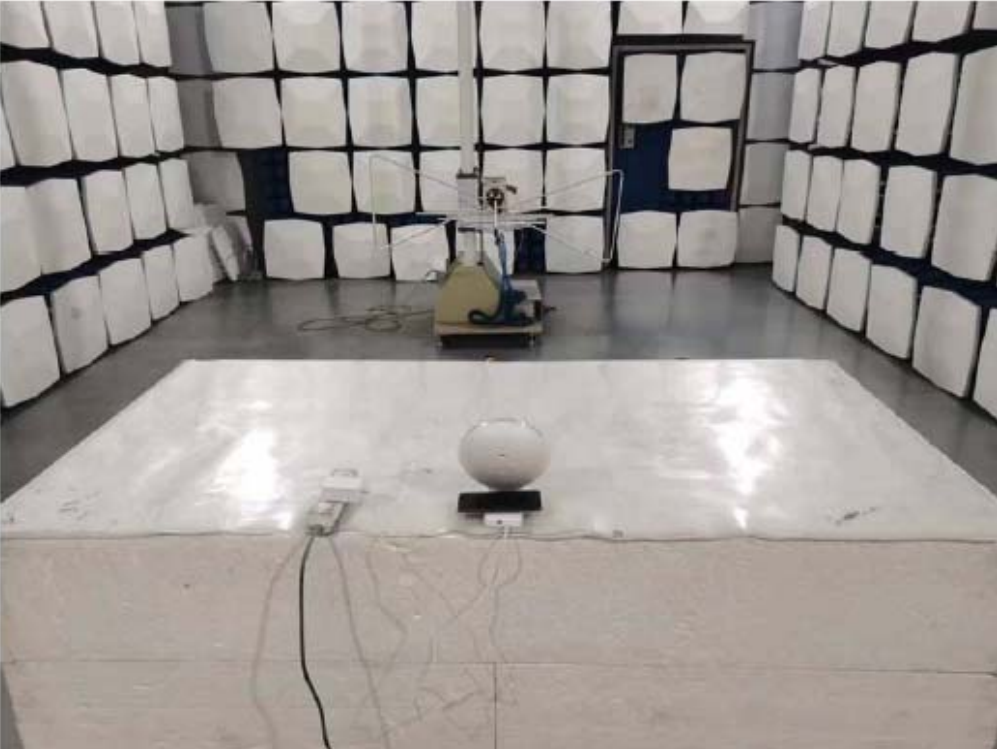
Radiated Emission Test Setup
