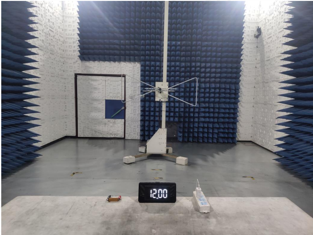
FCC RADIATED EMISSION TEST SETUP ABOVE 1GHZ
