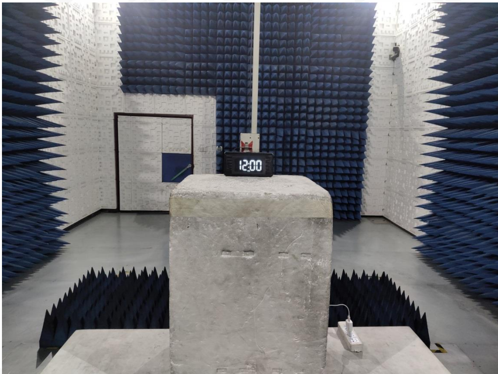
FCC RADIATED EMISSION TEST SETUP ABOVE 1GHZ
