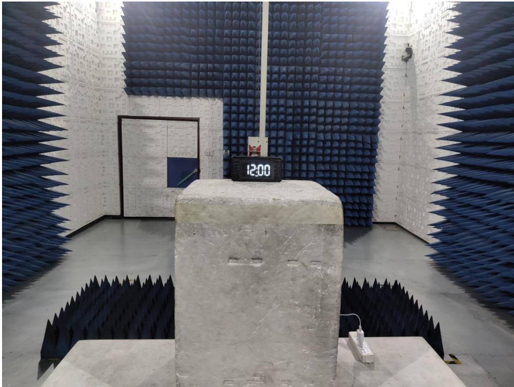
FCC RADIATED EMISSION TEST SETUP ABOVE 1GHZ
