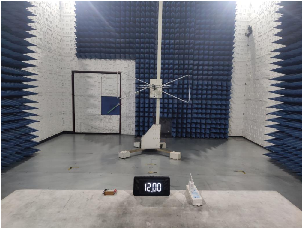
FCC RADIATED EMISSION TEST SETUP ABOVE 1GHZ
