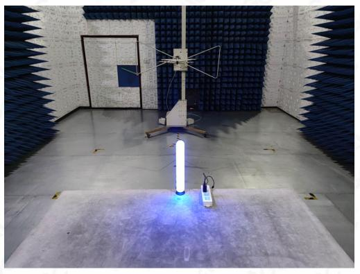
RADIATED EMISSION TEST SETUP ABOVE 1GHz
