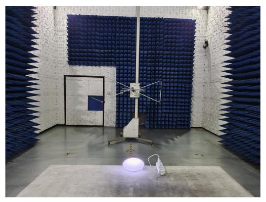
FCC RADIATED EMISSION TEST SETUP ABOVE 1GHZ
