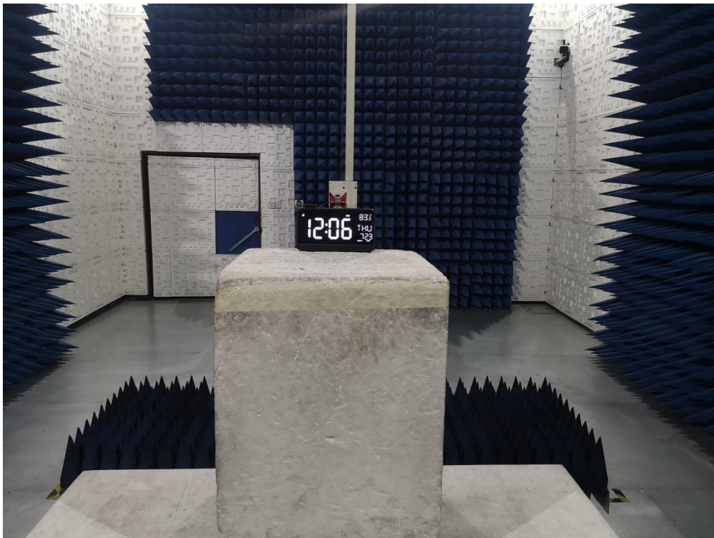
FCC RADIATED EMISSION TEST SETUP ABOVE 1GHZ
