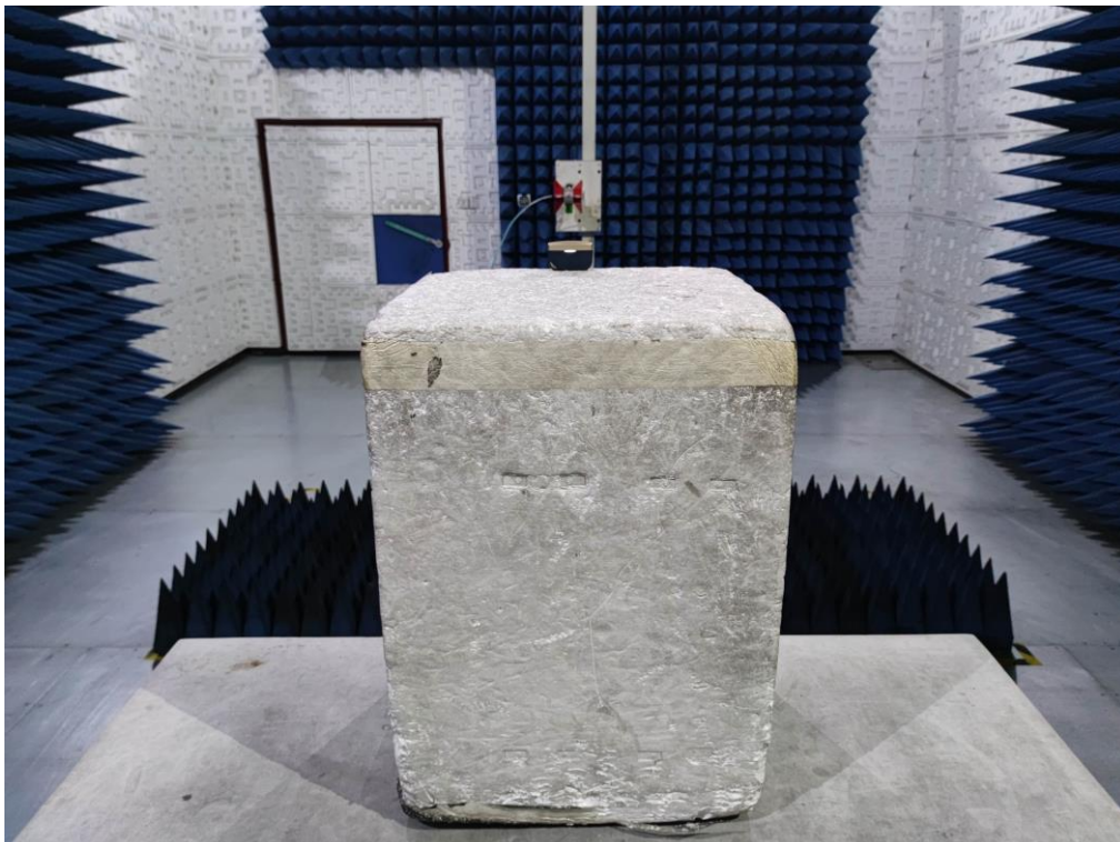
RADIATED EMISSION TEST SETUP ABOVE 1GHz
