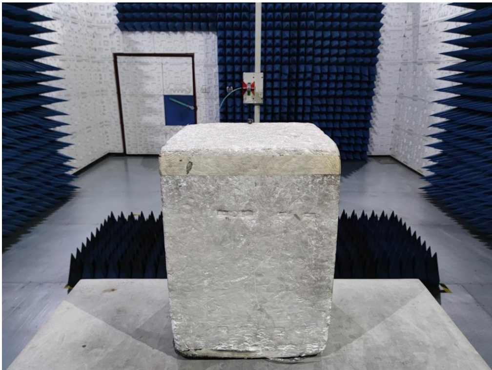
RADIATED EMISSION TEST SETUP ABOVE 1GHZ
