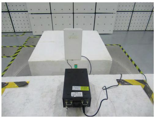
Description: Radiated Emission Test Setup for 110GHz ~ 140GHz
