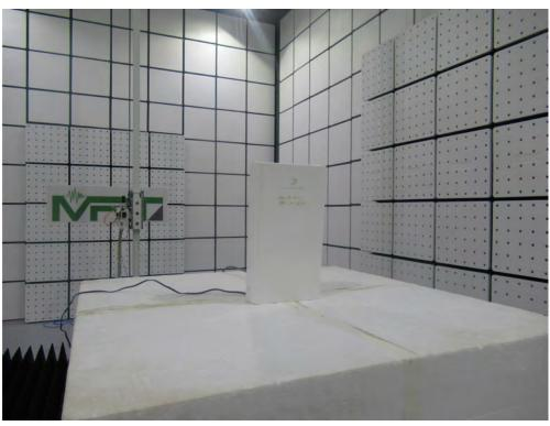
Description: Radiated Emission Test Setup for  $18GHz \sim 40GHz$
