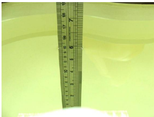
Fig 6.10 Photo of Liquid Height for Head SAR
