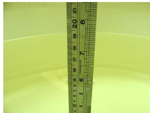
Fig 6.11 Photo of Liquid Height for Body SAR
