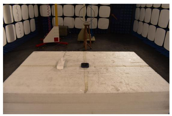
3. Radiated emission (9KHz-30MHz)
