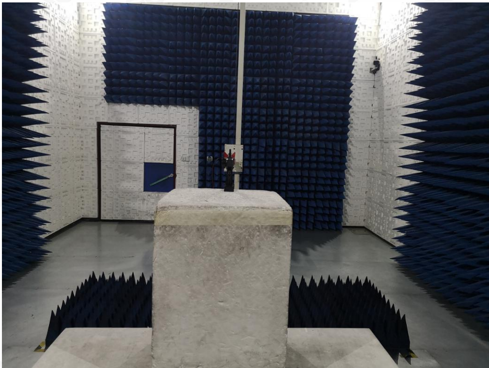
FCC RADIATED EMISSION TEST SETUP ABOVE 1GHZ
