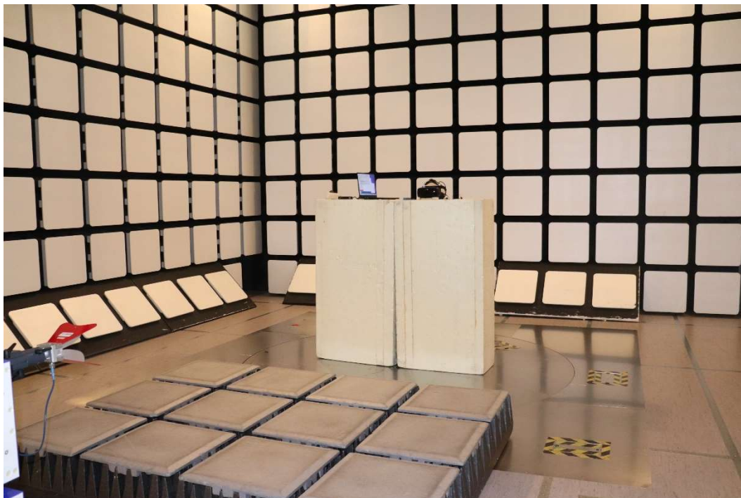
Photograph 5. Radiated emission test setup (1 GHz – 18 GHz)
