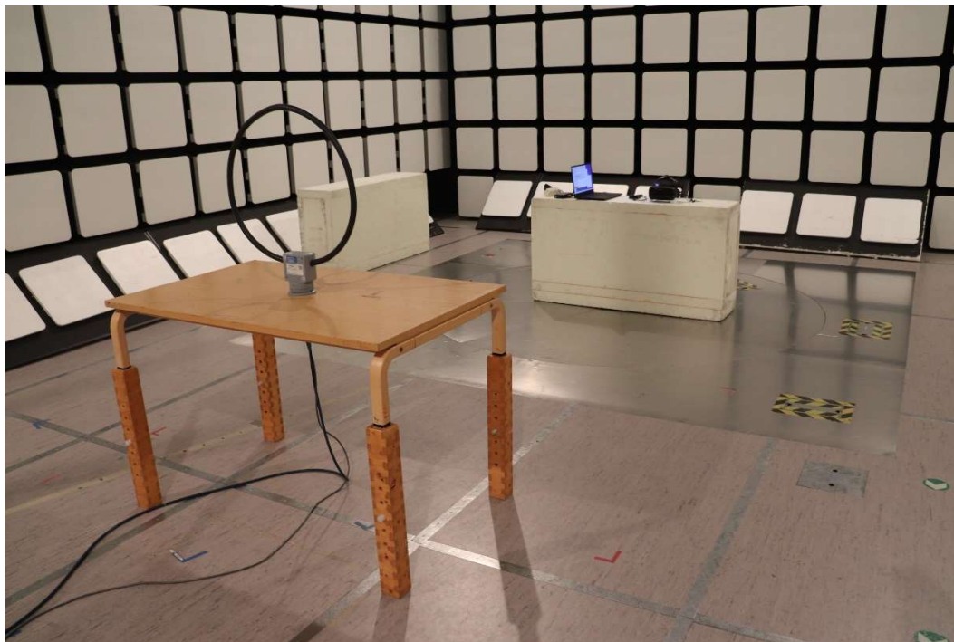
Photograph 3. Radiated emission test setup (9 kHz – 30 MHz)
