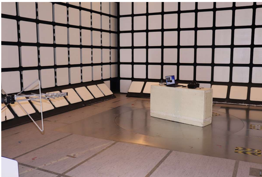
Photograph 4. Radiated emission test setup (30 MHz – 1000 MHz)
