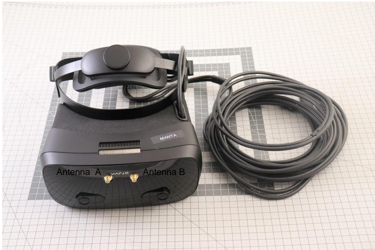
Photograph 2. The EUT2 with antenna connectors
