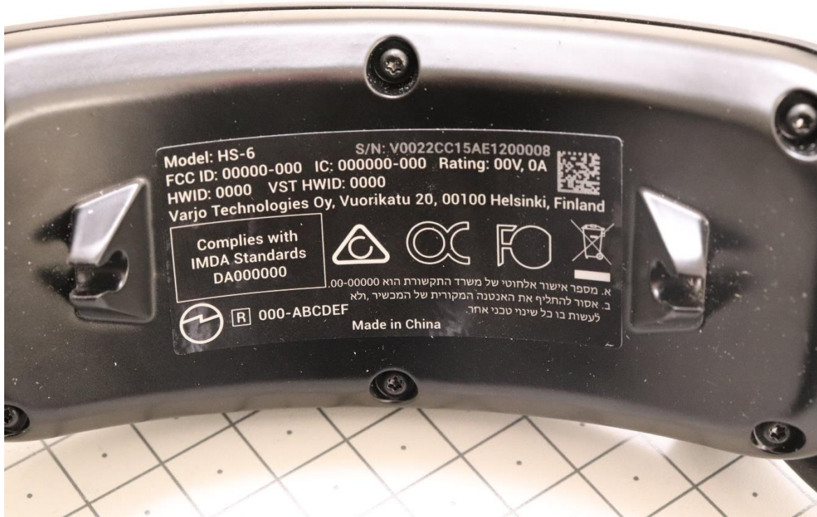
Photograph 5. The type label of the EUT1
