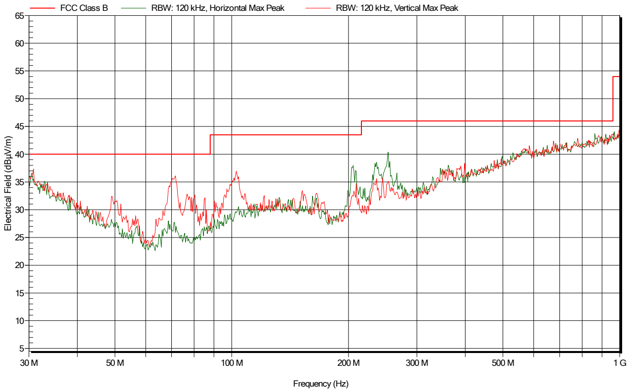
Figure 5.3.7.3: Electric field emissions Peak Detector Plot, 30MHz to 1GHz Operation on 2402MHz
