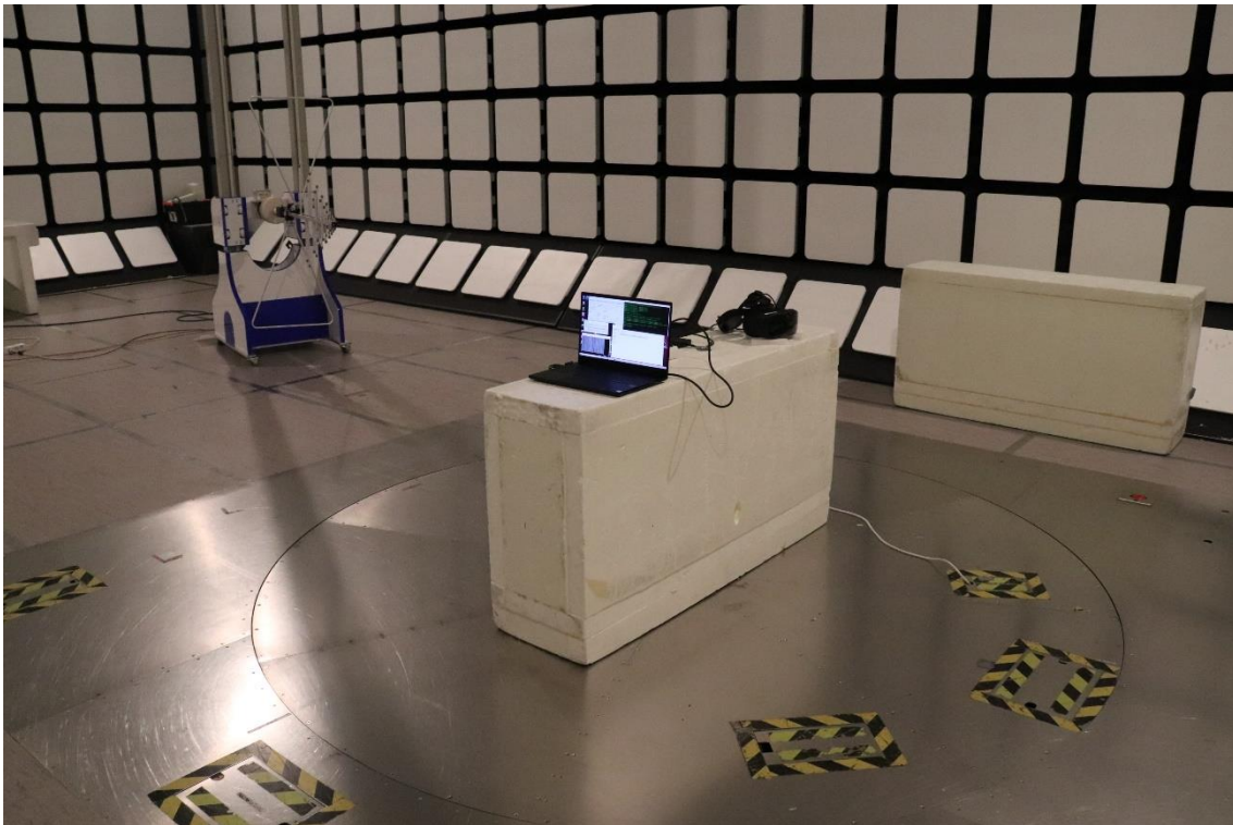
Photograph 3. Test setup for Radiated Emissions (30 – 1000 MHz)
