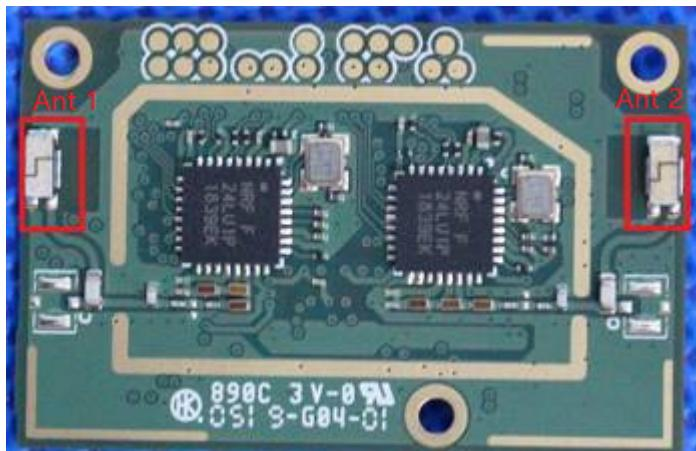
This two antennas is integrated on the main PCB and no consideration of replacement. The best case gain of the antenna is 0 dBi.
