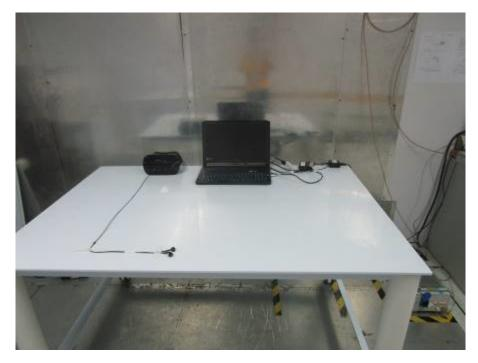
1.2 Radiated Emissions (30MHz-1GHz) Test Setup
