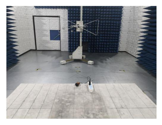
RADIATED EMISSION TEST SETUP ABOVE 1GHZ
