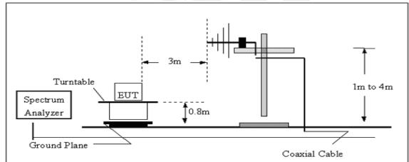
(C) Radiated Emission Test-Up Frequency Above 1GHz
