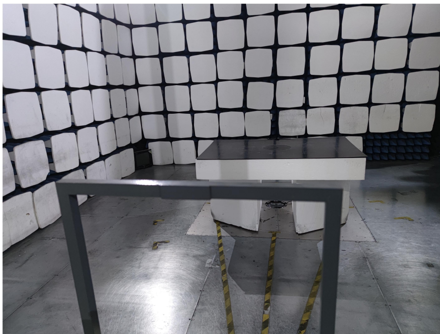
Radiation Emission Test Setup (Below 30MHz)
