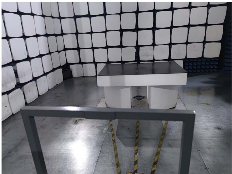
Radiation Emission Test Setup (Below 30MHz)
