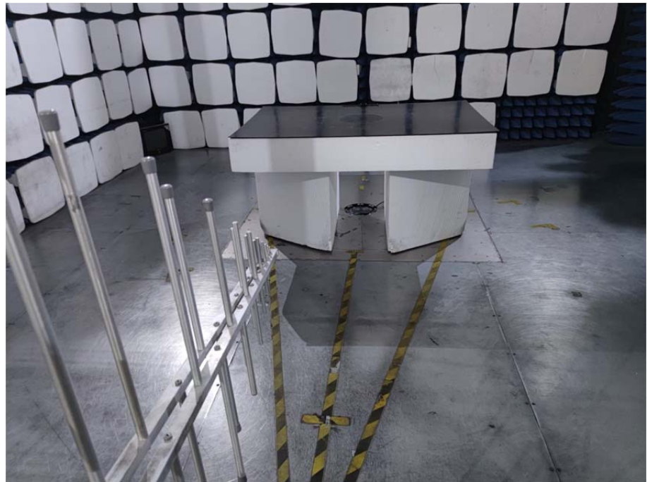
Radiation Emission Test Setup (30MHz to 1GHz)
