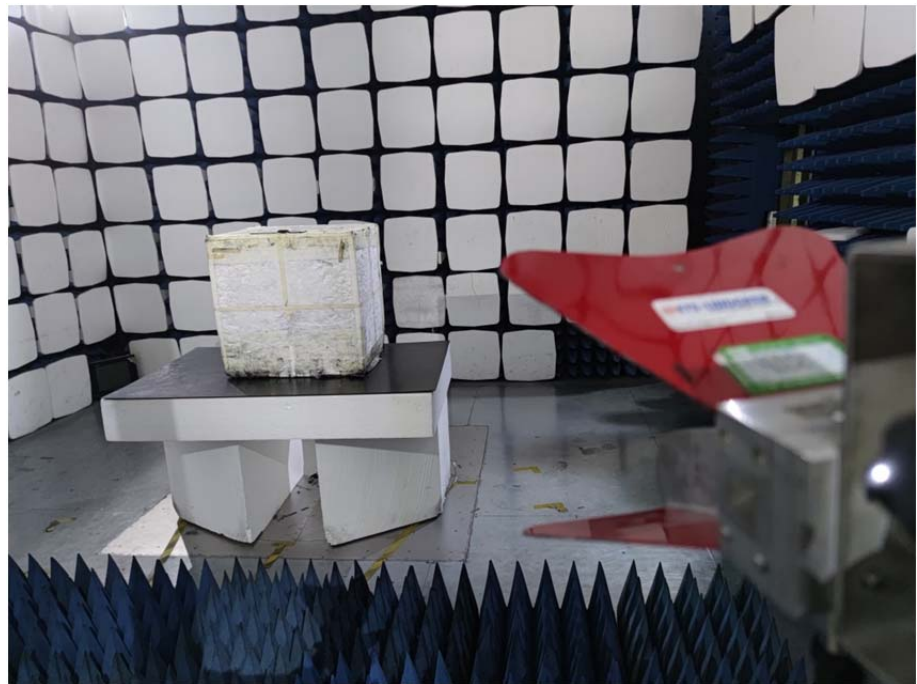
Radiation Emission Test Setup (1GHz to 18GHz)
