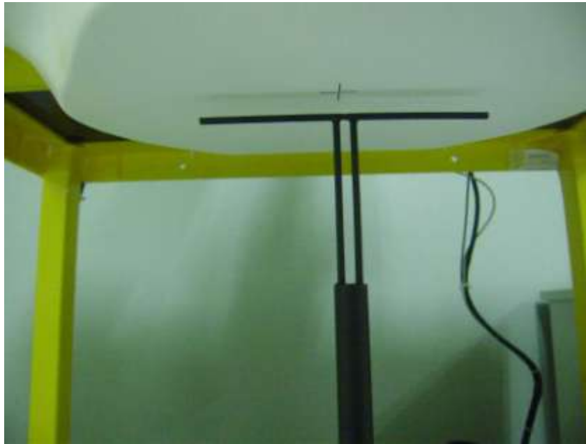
Setup Photo of Dipole Antenna
