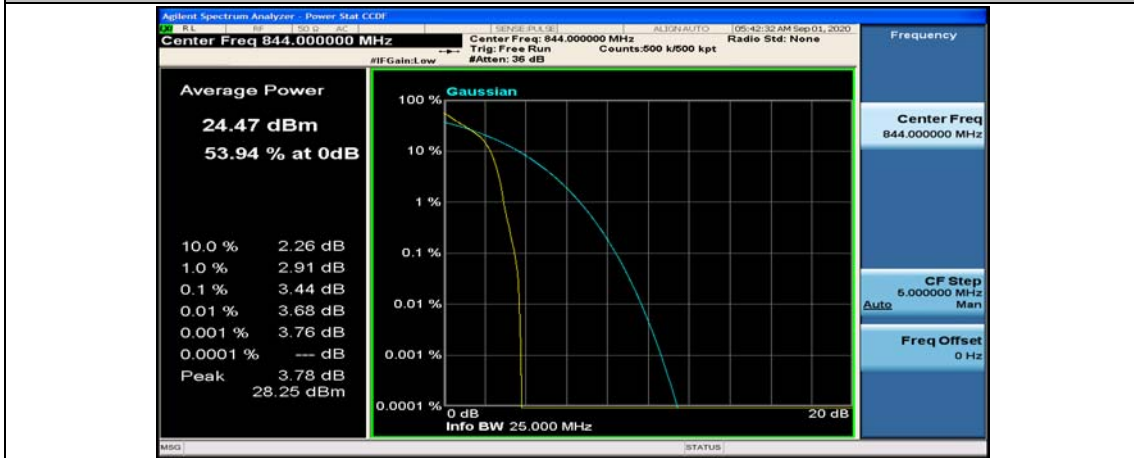
Channel Bandwidth: 10 MHz_HCH_QPSK_25RB#0
