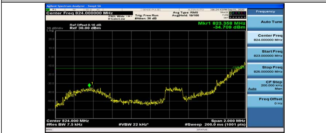
(Channel Bandwidth: 1.4 MHz)_LCH_16QAM_3RB#0
