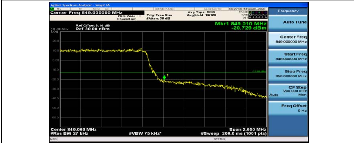
(Channel Bandwidth: 1.4 MHz)_HCH_QPSK_6RB#0
