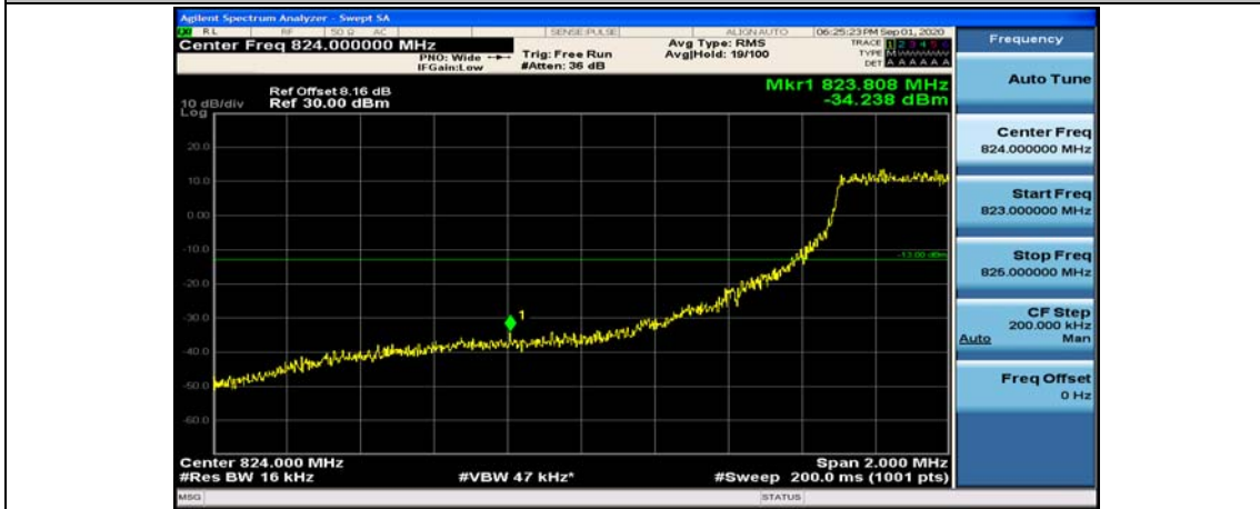
(Channel Bandwidth: 1.4 MHz)_LCH_16QAM_6RB#0
