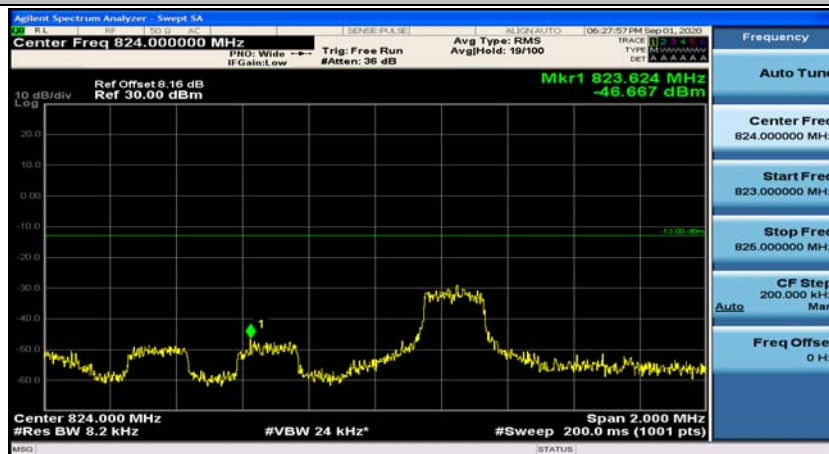
(Channel Bandwidth: 3 MHz)_LCH_16QAM_8RB#0
