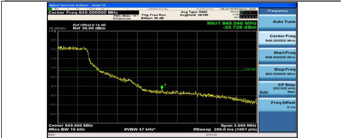
(Channel Bandwidth: 1.4 MHz)_HCH_16QAM_3RB#2
