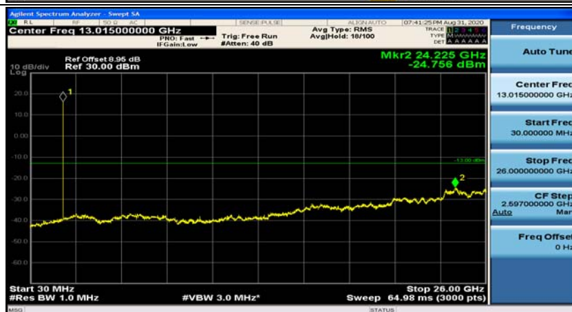
(Channel Bandwidth:15 MHz)_HCH_16QAM_1RB#37
