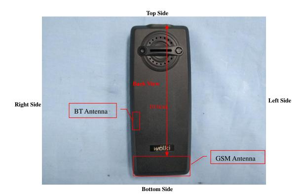
**Block Diagram for EUT Antenna Position**
