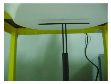
**Setup Photo of Dipole Antenna**
