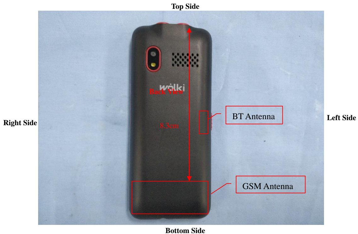
Block Diagram for EUT Antenna Position
