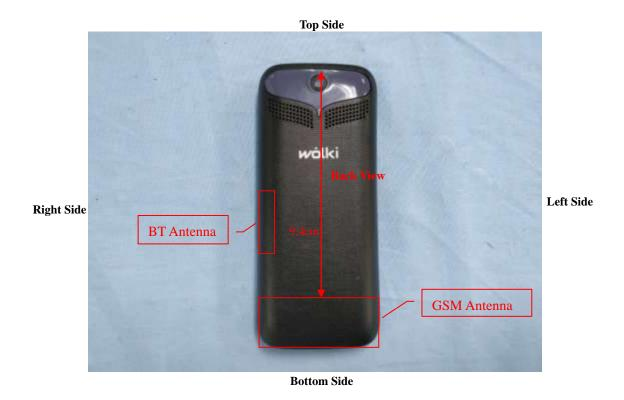
**Block Diagram for EUT Antenna Position**
