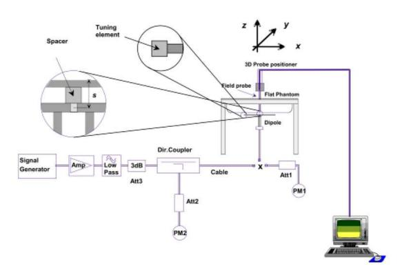
**System Verification Setup Block Diagram**
