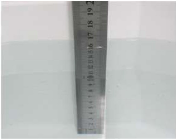
Liquid Height for Head SAR
