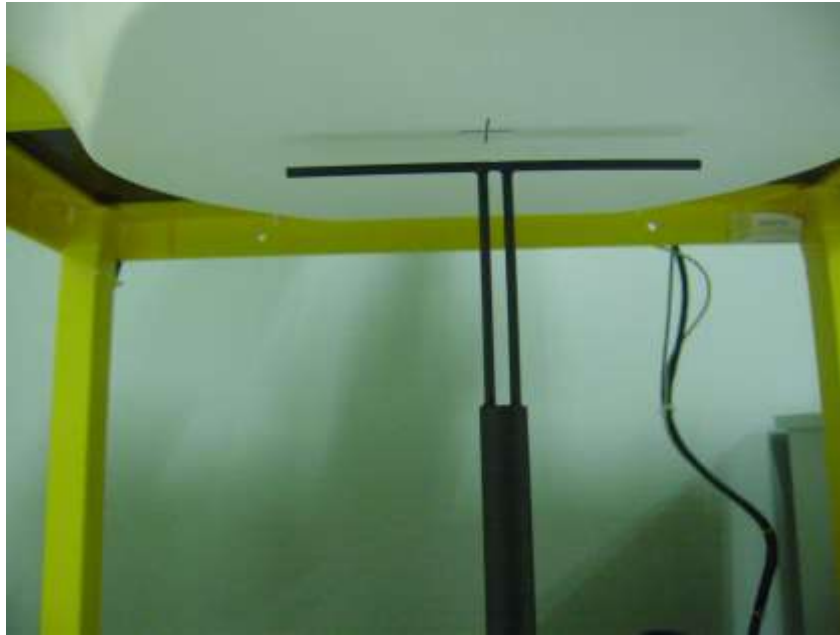
Setup Photo of Dipole Antenna
