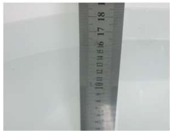
Liquid Height for Body SAR
