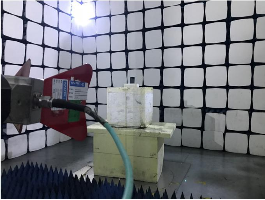
Radiation Emission Test Setup (1GHz to 18GHz)
