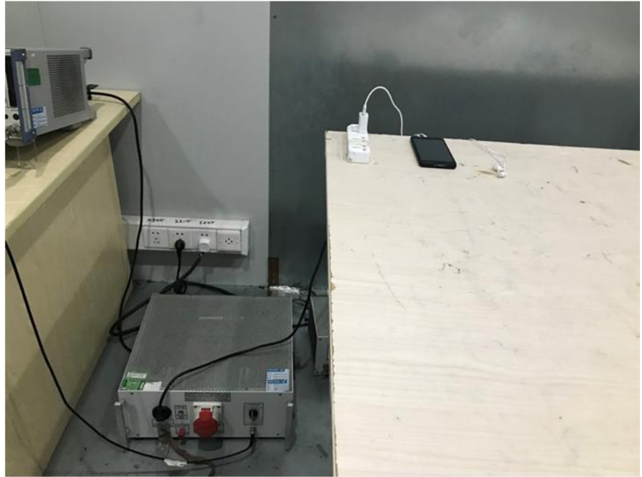
Conducted Emission Test Setup*
