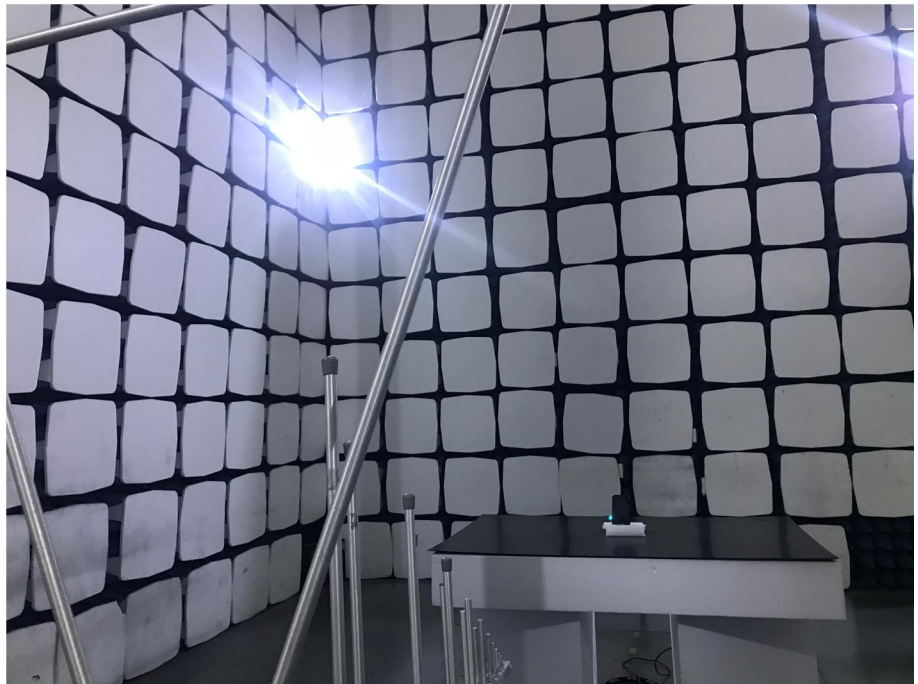
Radiation Emission Test Setup (30MHz to 1GHz)
