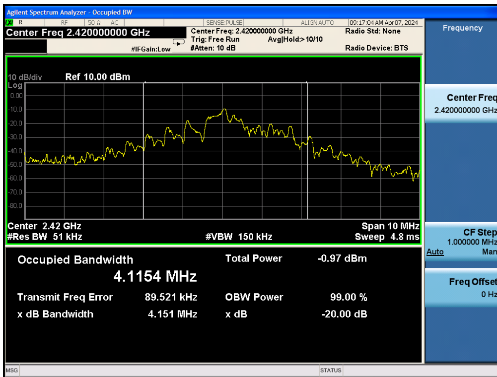
TEST PLOT OF BANDWIDTH FOR LOW CHANNEL
