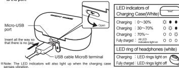
② Connect the other end to a booted computer. Connect the Type A terminal side of The USB cable to the USB port of a booted PC or USB AC adapter. (Commercially available, DC 5V.)
