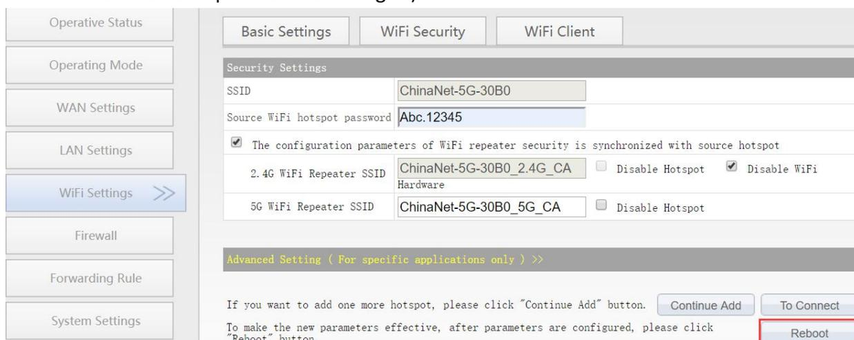
**Remark 3:** After VONETS module/WiFi product sets the WAN port to access the WiFi hotspot in the routing mode, its LAN port IP is still 192.168.254.254, and the terminal device also obtains the IP address of the same network segment, can login configuration page by 192.168.254.254 or <http://vonets.cfg>.
