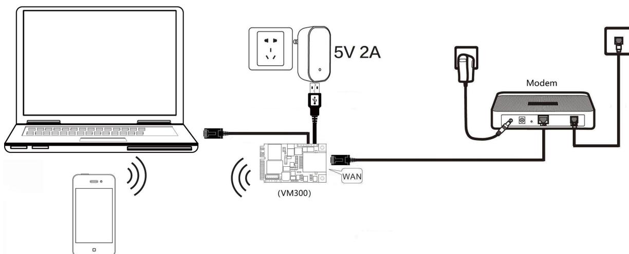
The Ethernet cable of **VM5G** module/**VBG1200** WiFi product defaults to LAN port, you must set “WAN/LAN interchange” so that the Ethernet cable is WAN port to use the broadband dialing function.
