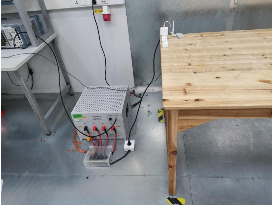
Photo of Power Line Conducted Emission Test
